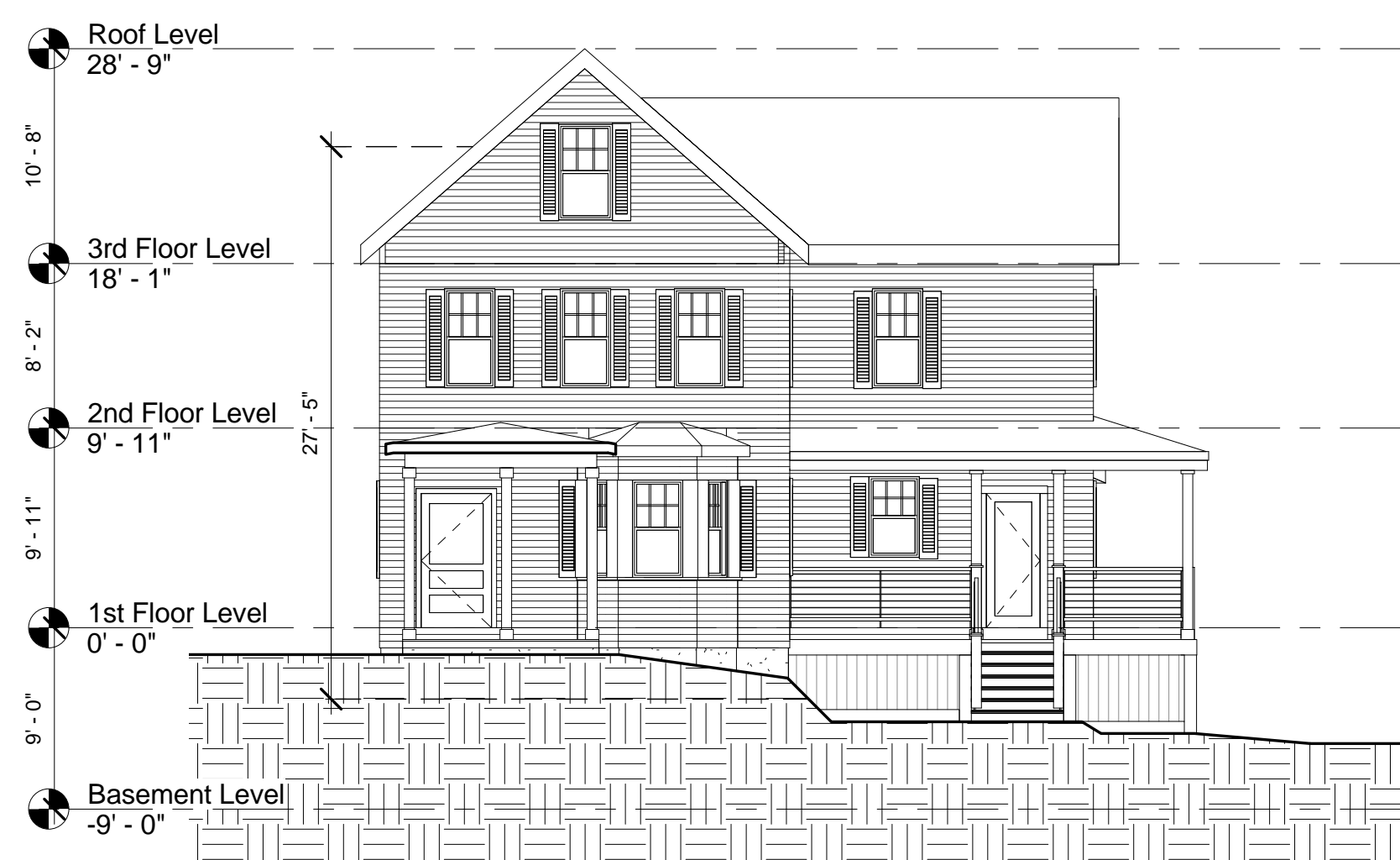
5 Existing East Elevation 1/8" = 1'-0"
